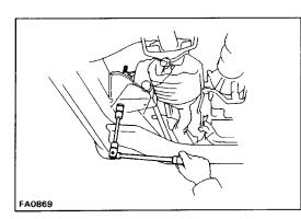
(d) Tighten the adjusting nut so that the bolt protrusion is equal to that before removal.
