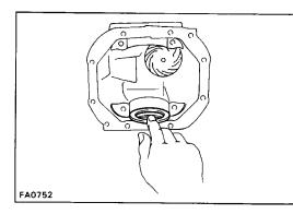
(f) Remove the plate washers and differential case.(g) Install the plate washer into the lower part of the carrier.
