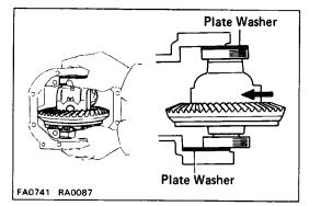
(h) Place the other plate washer onto the differential case together with the outer race, and install the differential case with the outer race into the carrier.
