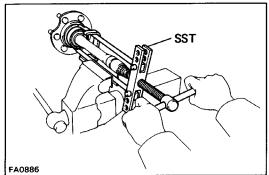
(b) Using SST, remove the bearing from the LH side gear shaft. SST 09950–20017
