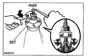
(c) Using SST, remove the companion flange. SST 09557–22022 (09557–22030)
