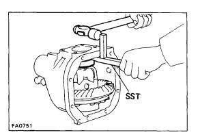
(c) Using SST and a hammer, remove the two side bearing preload adjusting plate washers. SST 09504-22011
