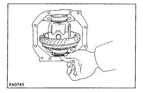
(d) Select a ring gear back plate washer, using the backlash as reference. (See page SA-77)
