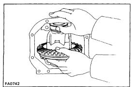
(e) Select a ring gear teeth side washer with a thickness which eliminates any clearance between the outer race and case.
