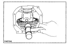
(b) Snug down the washer and bearing by tapping on the ring gear with a plastic–faced hammer.
