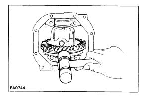
(i) Using a plastic–faced hammer, snug down the washer and bearing by tapping the ring gear.
