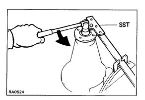
(b) Using SST to hold the flange, remove the nut. SST 09330–00021
