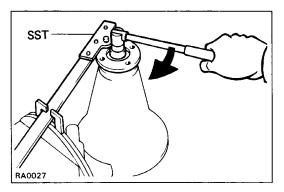
(e) Adjust the drive pinion preload by tightening the companion flange nut.
