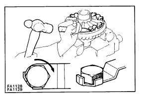
(h) Using a hammer and drift punch, stake the lick plates.
