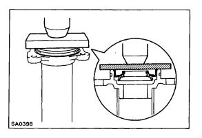
(b) With the oil seal lip facing upward, use press and plate to press in a new side oil seal until its end is flush with the surface of the tube.
