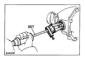
2. REPLACE SIDE OIL SEAL (a) Using SST, remove the oil seal. SST 09308–00010
