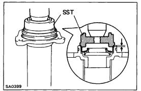
(c) Using SST, press in the oil seal. SST 09554–14010
