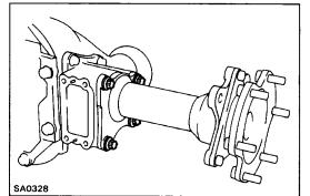
(c) Install the side gear shaft with tube.
