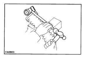
(c) Using a brass bar and hammer, remove the tripod joint from the drive shaft.
