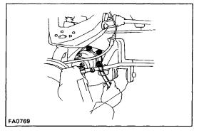
(b) Temporarily install the six nuts.
