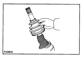
6. REMOVE OUTBOARD JOINT BOOT CLAMPS AND BOOT NOTICE: Do not disassemble the outboard joint.
