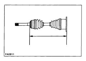
(c) Insure that the boot is not stretched or contracted when the drive shaft is at standard length.
