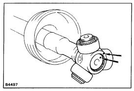
(b) Align the matchmarks placed before disassembly.
