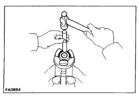
(e) Using a brass bar and hammer, tap in the tripod joint to the drive shaft.
