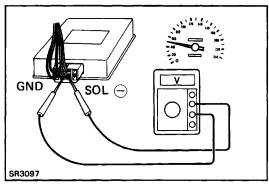
(b) Place the transmission in gear and while running at about 50 km/h (31 mph), measure the voltage be tween the ECU terminals GND and SOL E). Standard voltage: Voltage measured in (a) above, plus 0.12 – 0.24 V If no voltage, try another ECU.
