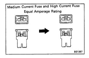
When replacing fuses, be sure the new fuse has the correct amperage rating. DO NOT exceed the rating or use one with a lower rating.
