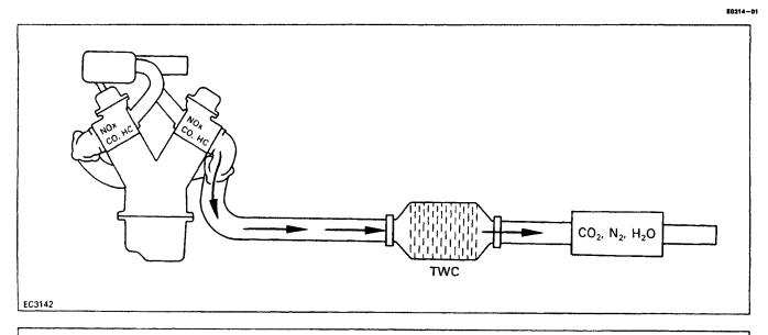
To reduce HC, CO and NOx emissions, they are oxidized, reduced and converted to nitrogen (N<sub>2</sub>), carbon dioxide (CO<sub>2</sub>) and water (H<sub>2</sub>) by the catalyst.
