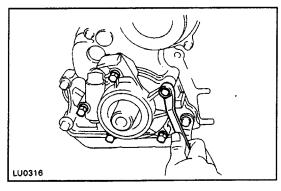
(b) Remove the five bolts, the oil pump assembly and O-ring.
