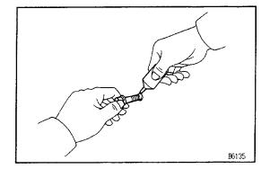
(b) Apply sealant to 2 or 3 threads of the bolt end.
