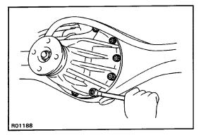
(c) Remove the differential carrier assembly.
