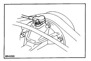
(e) Install the differential carrier assembly. (See page SA-151 )
