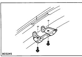
8. INSTALL REMOVABLE ROOF LOCK BASE Install the lock base, and lightly tighten the bolts.
