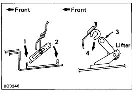
7. INSTALL WIND DEFLECTOR PANEL Install the deflector clips as shown in the illustration.
