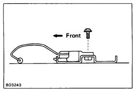
6. INSTALL REMOVABLE ROOF AUXILIARY CATCH Install the auxiliary catch with the bolt.
