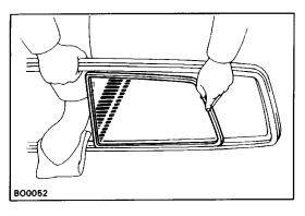
(b) Pull apart the channels and remove two non–slide glass panes as shown.
