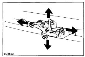
**6. ADJUST HOOD LOCK** Adjust the lock by loosening the bolts.
