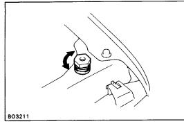
2. ADJUST FRONT EDGE OF HOOD IN VERTICAL DIRECTION
