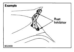
2. If a hinge or exterior body panel is loosened or removed, be sure apply rust inhibitor after repairs.
