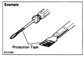
2. When prying off the body parts with a screwdriver or scraper etc., be sure to apply protection tape to the tip or blade to prevent damage to the paint film or body part.
