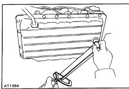
(b) Install the oil strainer case and torque the five bolts. Torque: 10 N–m (100 kgf–cm, 7 ft–lbf )
