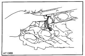
(b) Disconnect the throttle cable from the cam and remove the valve body. INSTALLATION OF VALVE BODY **1. CONNECT THROTTLE CABLE TO CAM** Push the cable fitting into the cam.
