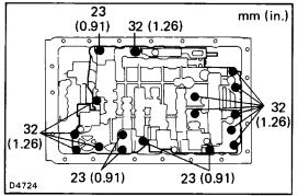
(b) Finger tighten the all bolts first. Then tighten the bolts evenly.
