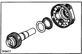
25. REMOVE INPUT SHAFT, THRUST BEARING AND RACE
