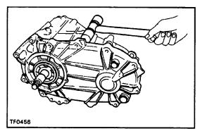
(b) Using a plastic hammer, tap the rear case and separate the front case and rear case.
