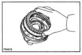
(b) Remove the low gear spline piece.
