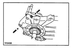
(b) Using a magnetic finger, remove the spring and ball from both holes.
