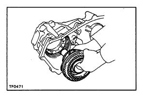
(b) Pull out the planetary gear assembly with the input shaft.
