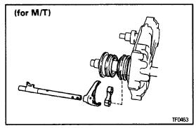
15. REMOVE HIGH AND LOW FORK SHAFT, FORK AND STOPPER
