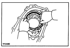
(c) Remove the planetary ring gear.
