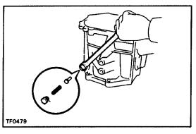
(b) Remove the plug, spring and pin.
