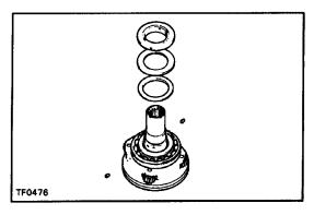
(b) Remove the input shaft stopper, thrust bearing, race and the 2 pins.
