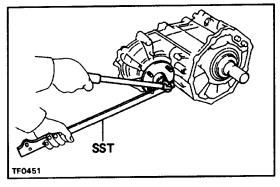
(b) Using SST to hold the flange, remove the companion flange lock nut.
