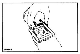
(b) Remove the select return spring from the retainer.
