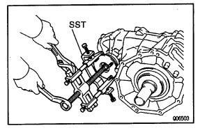
(c) Using SST, remove the companion flange. SST 09950–40010
