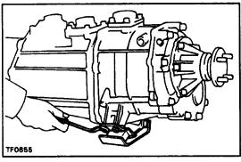
2. INSTALL ENGINE REAR MOUNTING
