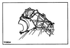
(e) Install and torque the bolts with the propeller shaft upper dust cover.
