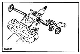
8. REMOVE TILT LEVER ASSEMBLY, TILT LEVER, TILT SUB LEVER AND TILT LEVER LOCK SHAFT
