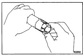
(b) Align the projections on a new bushing with the holes in the column lower tube. Install the bushing until the projections are firmly engaged in the holes in the tube.
