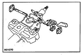
6. INSTALL TILT LEVER LOCK SHAFT, TILT SUB LEVER, TILT LEVER, AND TILT LEVER ASSEMBLY
