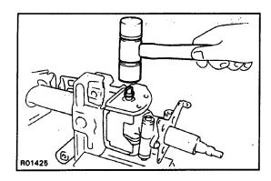
(c) Using a plastic hammer, drive in the 2 tilt No.2 bolts.
