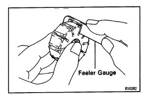
(b) Using a feeler gauge, measure the clearance between the rotor groove and vane plate.
