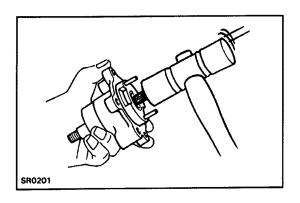
(c) Using a plastic hammer, tap out the rotor from the front housing.
