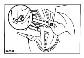
(c) Install the lateral control rod to the frame with the bolt, washer and nut.
