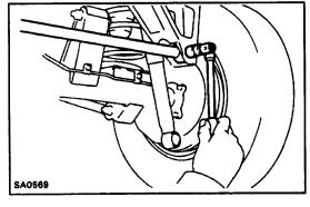
(b) Remove the nut, washer and bolt from the frame and disconnect the lateral control rod.
