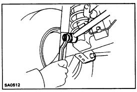
(c) Remove the nut, washer and bushings from the rear axle housing, and remove the lateral control rod.
