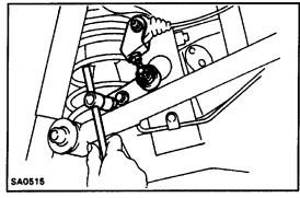
(d) Connect the shackle bracket to the lateral control rod with the 2 bolts.
