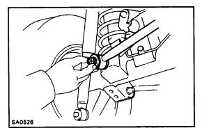
(b) In this order, install the bushing, lateral control rod, bushing, washer and nut on the rear axle housing.HINT: Do not tighten the nut.
