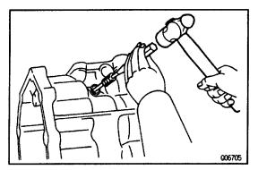
(b) Using a pin punch and hammer, drive out the slotted spring pin.
