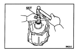
(b) Using SST and a hammer, drive in a new oil seal. SST 09325–12010
