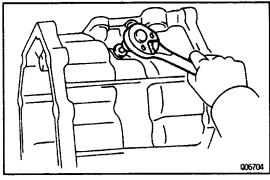
(c) Apply sealant to the plug threads.
