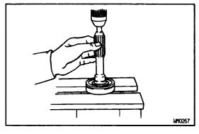
(b) Using a press, remove the bearing.
