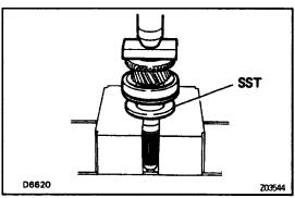
(c) Using SST and a press, install a new bearing. SST 09506 –35010
