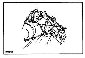
(e) Install and torque the bolts with the propeller shaft upper dust cover.
