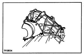
(c) Pull the transfer straight up and remove it from the transmission.
