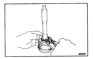
(e) Using a snap ring expander, install the snap ring.
