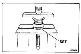
(c) Using SST and a press, install a now bearing. SST 09506–35010
