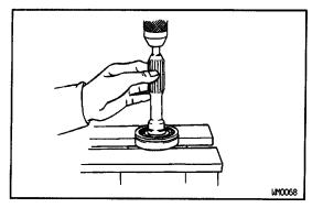
(b) Using a press, remove the bearing.
