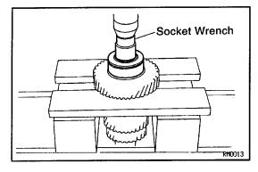
(d) Using a socket wrench and press, install a new bearing, the side race and inner race.
