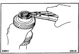
(f) Using a snap ring expander, install the snap ring.
