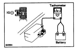
2. With a tachometer connected to the system, connect the tachometer test probe to the IG(–) terminal of the DLC 1.
