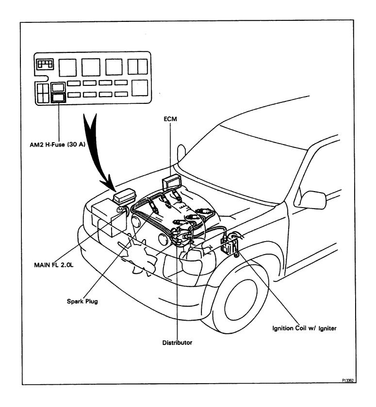
The ECM monitors the engine condition by signals from each sensor, calculates the ignition timing and sends an ignition signal to the igniter. High voltage from the ignition is distributed to each spark plug in the appropriate order to generate a spark between the electrodes, which ignites the air–fuel mixture.
