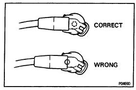
NOTICE: Check that the holder is correctly installed to the grommet and distributor cap a: shown in the illustration.
