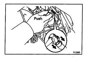
(b) Align the spline of the distributor (ignition coil) with the spline of the holder, and push in the cord.
