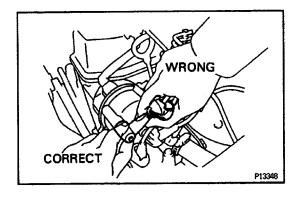
(b) Disconnect the high-tension cord at the grommet. DO NOT pull on the cord.
