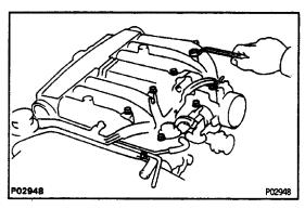
(p) Remove the 6 bolts, 2 nuts, intake chamber and gasket.
