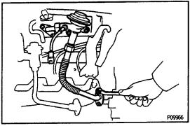
(I) Remove the 5 nuts, EGR valve with the pipes and 2 gaskets.
