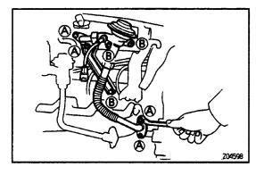
(h) Install the air intake chamber stay and throttle cable bracket. Install and torque the 6 nuts and 2 bolts.
