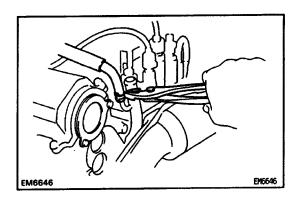
(e) Disconnect the No.5 water bypass hose from the water bypass pipe.
