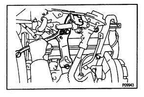
(k) Remove the nut, 2 bolts, intake chamber stay and throttle cable bracket.
