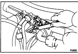
(n) Install the No.5 water bypass hose to the water bypass pipe.
