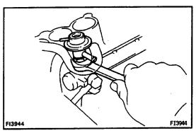
(e) Torque the lock nut.
