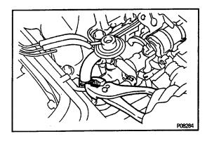
(o) Connect the No.4 water bypass hose to the union of the intake manifold.
