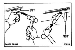
HINT: When removing the oil pan, be careful not to damage the oil pan flange.
