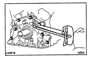
(e) Install the oil pump with the 7 bolts.
