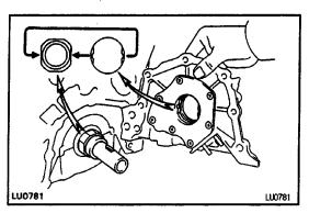
(d) Install the oil pump to the crankshaft with the spline teeth of the drive rotor engaged with the large teeth of the crankshaft.
