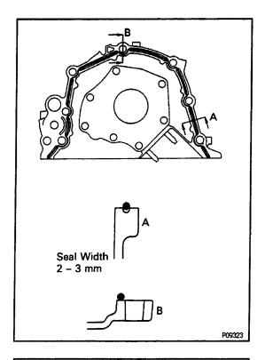
(b) Apply seal packing to the oil pump as shown in the illustration. **Seal pecking:**
