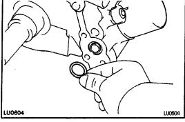
(c) Place a new O-ring into the groove of cylinder block.
