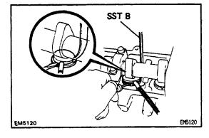
Remove the adjusting shim with a small screwdriver and magnetic finger.
