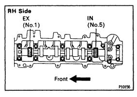
(f) Turn the crankshaft 1/3 revolution (120°), check the clearance of the IN (No.5) and EX (No-1) valves. Measure the valve clearance.
