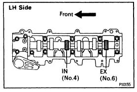
(e) Turn the crankshaft 1/3 revolution (120°), check the clearance of the IN (No.4) and EX (No.6) valves. Measure the valve clearance.
