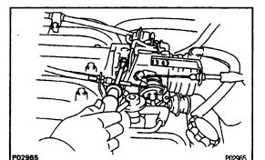
(c) Adjust the idle speed by turning the idle speed adjusting screw
