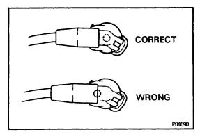
NOTICE: Check that the holder is correctly installed to the grommet and distributor cap a: shown in the illustration.
