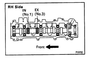
(b) Turn the crankshaft 1/3 revolution (120°), check the clearance of the IN (No.1) and EX (No.3) valves. Meas me the valve clearance.
