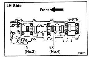
(c) Turn the crankshaft 1/3 revolution (120°), check this clearance of the IN (No.2) and EX (No.4) valves. Meas me the valve clearance.
