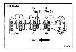
(d) Turn the crankshaft 1/3 revolution (120°), check the clearance of the IN (No.3) and EX (No.5) valves.
