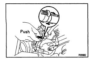
(b) Align the spline of the distributor (ignition coil) with the spline of the holder, and push in the cord.
