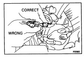
(b) Disconnect the high–tension cord at the grommet. DO NOT pull on the cord.
