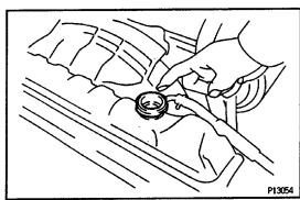
(b) There should not be any excessive deposits of rust or scale around the radiator cap or radiator filler hole, and the coolant should be free from oil.
