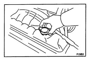
(c) Reinstall the radiator cap.
