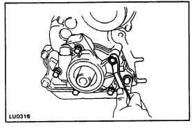
(b) Remove the 5 bolts, the oil pump assembly and O-ring.
