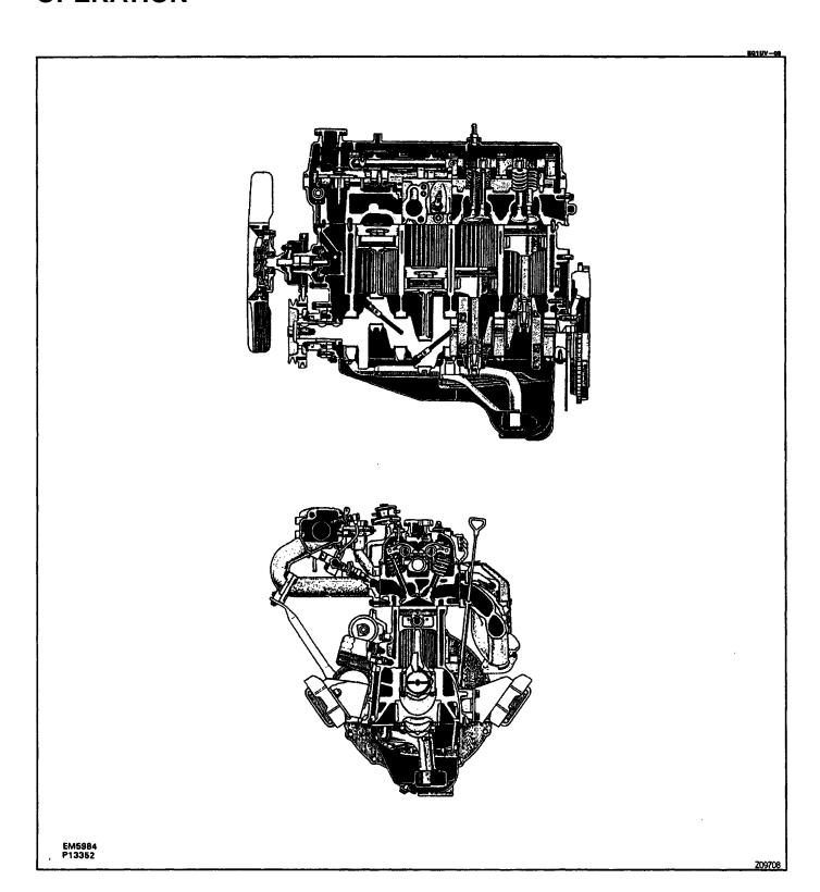
The 22R–E engine is in–line 4–cylinder engine with the cylinders numbered 1–2–3–4 from the front. The crankshaft is supported by 5 aluminium alloy bearings.
