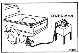
4. INSERT CO/HC METER TESTING PROBE AT LEAST 40 cm (1.3 ft) INTO TAILPIPE DURING IDLING 5. IMMEDIATELY CHECK CO/HC CONCENTRATION AT IDLE AND/OR 2.500 RPM
