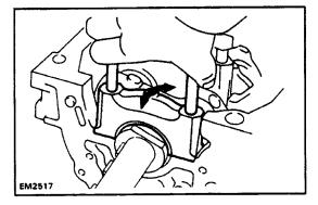
(b) Using the removed crank shaft bearing cap bolts, pry
