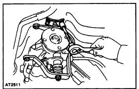
(c) Connect the No.1 and No.2 transfer shift linkage to the cross shaft.
