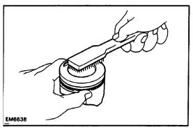
(c) Using solvent and a brush, thoroughly clean the piston.
