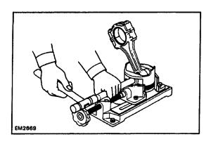
(c) Using a plastic–faced hammer and brass bar, lightly tap out the piston pin from the piston.
