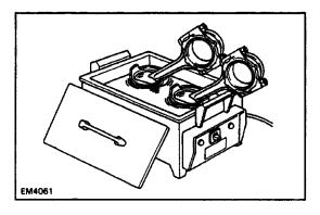
(b) Heat the piston in hot water approx. 60°C(140°F).
