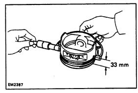
(a) Using a micrometer and with the piston upside down, measure the piston diameter at right angles to the piston pin hole center line, at the indicated distance from the piston head.
