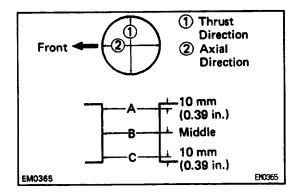
(b) Measure the cylinder bore diameter in thrust directions (See page EG –xx) and subtract the piston diameter measurement from the cylinder bore diameter measurement.
