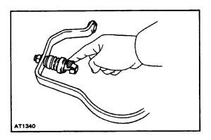
(b) install the cross shaft to the body.
