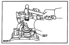
(b) Using SST and a hammer, tap in the oil seal until its surface is flush with the timing chain cover edge.
