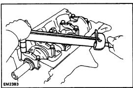
(h) Install the main bearing caps with the front mark facing forward. Install and torque the cap bolts.
