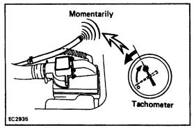
(c) Race the engine and quickly close the throttle valve Check that a bubbling noise stops momentarily.
