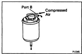
(b) Blow low pressure compressed air 4.71 kPa (48 gf/cm2, 0.68 psi) into port B and check that air does not flow from the other ports.
