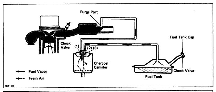
To reduce HC emission, evaporated fuel from the fuel tank is routed through the charcoal canister to the throttle body for combustion in the cylinders.
