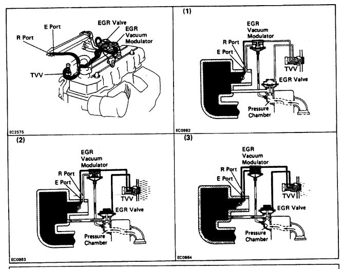
To reduce NOx emission, part of the exhaust gases are recirculated through the EGR valve to the intake manifold to lower the maximum combustion temperature.
