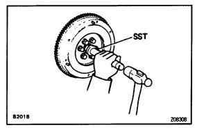
(b) Using SST and a hammer, install the pilot bearing. SST 09304–30012
