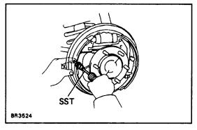
(b) Using SST, remove the shoe hold–down spring, cups and pin.
