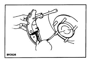
(c) Install the adjusting lever spring.
