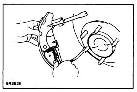
(c) Remove the adjusting lever spring.
