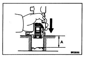
(c) Place a rag and 2 wooden blocks on the work table, and lightly tap the cylinder flange against the block edges until the No.2 piston drops out of the cylinder. HINT: Make sure the distance (A) from the rag to the
