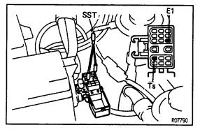
(b) Check that the warning light blinks about 4 times every second from 3 seconds after the engine is started.
