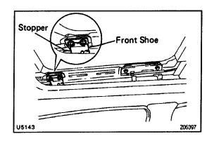
HINT: When the sliding roof is fully closed, confirm that the front shoes are in contact with the stopper.
