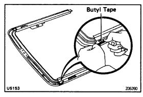
(c) Use butyl tape to cover the cut portion of the weatherstrip at the connection between the guide casing and guide rail.
