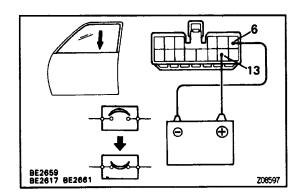
(d) Reverse the polarity, check that the window begins to descend within approximately 60 seconds.If operation is not as specified, replace the motor.
