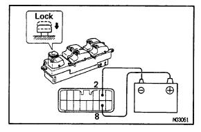
(c) Set the window lock switch to the lock position, check that all the passenger's power window switch illuminations go out.
