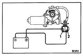
(b) Connect the positive (+) lead from the battery to terminal 1 and the negative (-) lead to terminal 2 and check that the motor turns counterclockwise.
