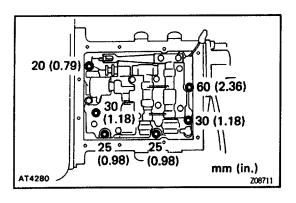
(b) Install the bolts, as shown. Torque the bolts evenly. Torque: 10 N-m (100 kgf-cm, 7 ft-lbf)
