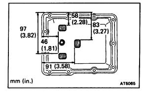
(c) Install the 3 magnets, as shown.
