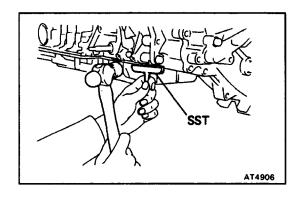
(b) Install the blade of SST between the transfer case and oil pan, cut oft applied sealer.
