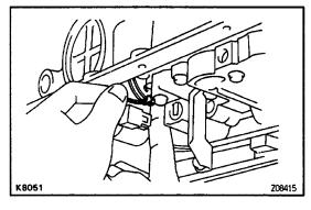
2. CONNECT THROTTLE CABLE TO VALVE BODY Connect throttle cable to the cam.
