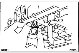
7. DISCONNECT THROTTLE CABLE FROM VALVE BODY
