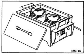
(b) Heat the piston in hot water to approx. 80°C (176°F).
