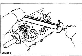
(g) Align the rod and cap marks and fit on the cap. Install and torque the cap nuts.
