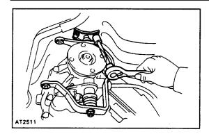
(b) Remove the cross shaft from the body.
