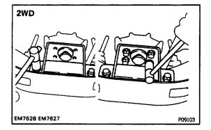
(b) Install the engine rear mounting bracket to the support member. Torque the 2 bolts.
