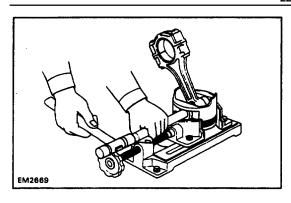
(c) Using a plastic-faced hammer and brass bar, lightly tap out the piston pin from the piston.
