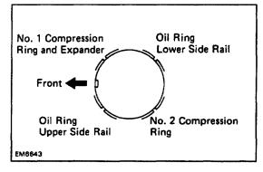
(c) Position the piston rings so that the ring end gaps are as shown.
