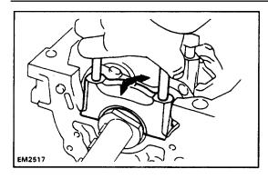
(b) Using the removed bearing cap bolts, pry the bearing cap fore and aft, and remove it with the lower bearing and (No.3 journal only) thrust washers.
