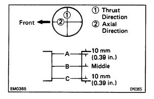
Measure the cylinder bore diameter in thrust directions (See page EG1-58) and subtract the piston diameter measurement from the cylinder bore diameter measurement.
