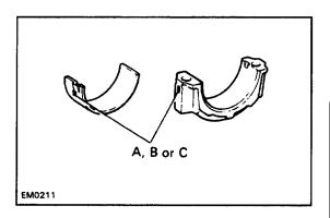
HINT: If replacing a standard size bearing, replace with one having the same letter as marked on the bearing cap. There are 3 sizes of standard bearings supplied, marked A, B or C respectively.
