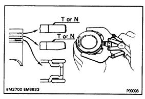
(b) Using a ring expander, install the 2 compression rings with the code marks facing upward.
