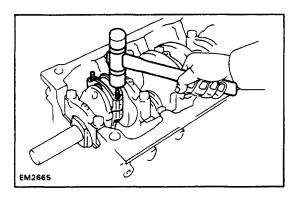
(c) Using a plastic-faced hammer, tap the rod bolts lightly and lift off the rod cap.
