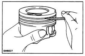
(b) Using a groove cleaning tool or broken ring, clean the ring grooves.
