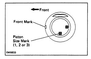
2. INSPECT PISTON DIAMETER AND OIL CLEARANCE
