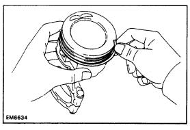
(b) Remove the 2 side rails and oil ring expander by hand. HINT: Keep the rings for each cylinder separated.
