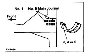
HINT: If using a standard bearing, replace with one having the same number as marked on the cylinder block. There are 3 sizes of standard bearings, marked 3, 4, 5 accordingly.
