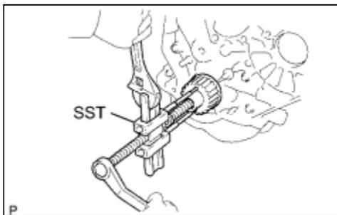
(a) Remove the crankshaft timing pulley.
