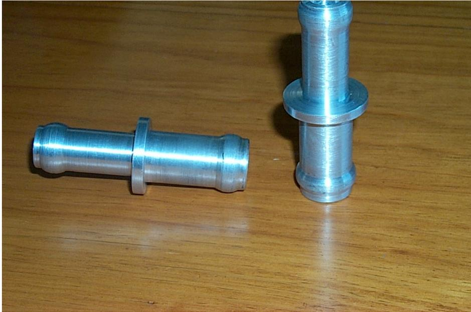
I had a friend turn up two reducers on his lathe. They were made from aluminium and allow the connection of a 19mm ID pipe to a 16mm ID pipe. These items may be available off the shelf but I am not aware of a source.
