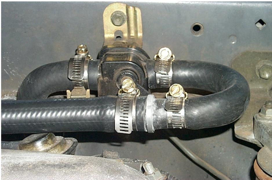
From the hose parts bin in the local car accessories store I bought a 16mm ID pipe with a “U” bend in it to connect to the tap. This then allowed me to run from the reducer via the original hose bracket to the motor takeoff pipes. In changing the pipes I removed completely the hoses and pipe work to the centre console heater box as I had no use for it.
