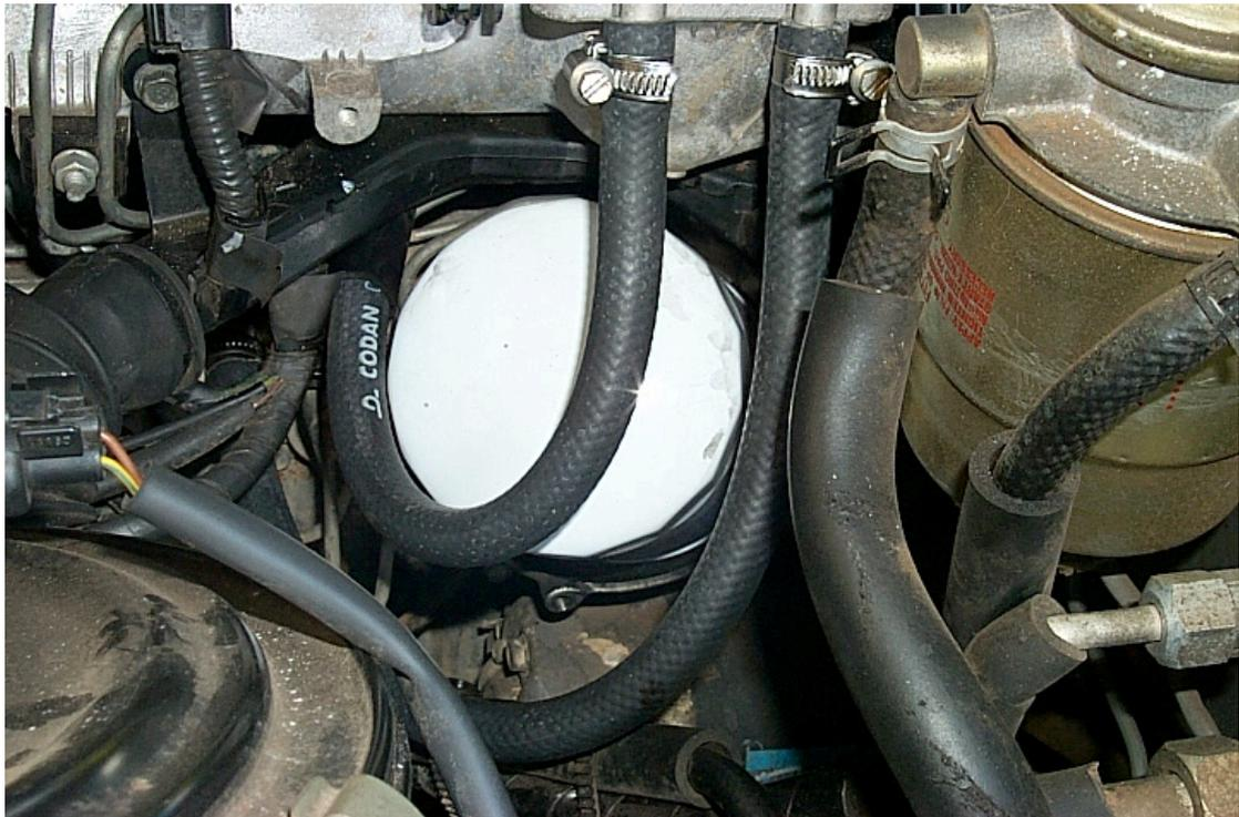
Again genuine hoses were not available for the pipes to the throttle body. I have sleeved the pipes to avoid damage from rubbing and have left enough slack to replace the oil filter.
